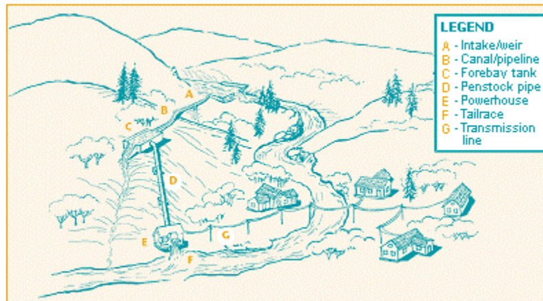
Figure 2. Principal components of a micro-hydropower system
